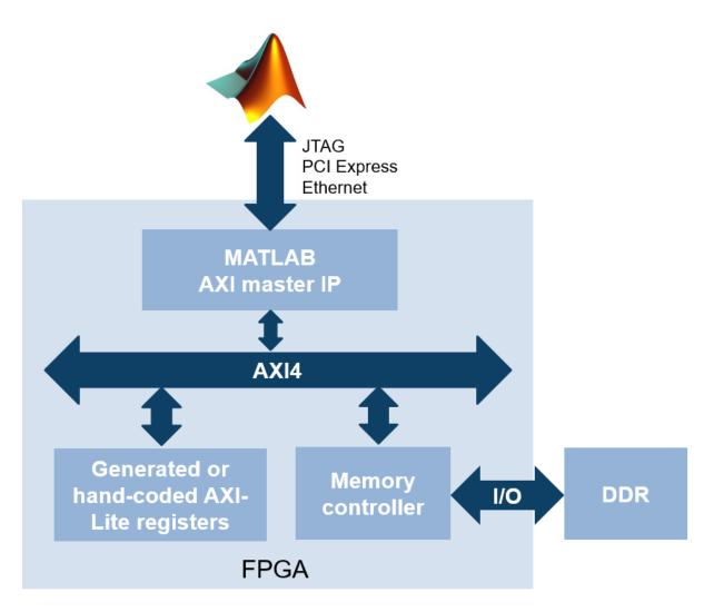
To set up the AXI master IP for access from MATLAB, follow these setup steps:
