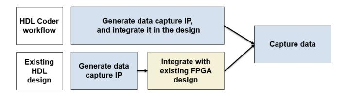
To capture signals from your design, HDL Verifier generates an IP core that communicates with MATLAB. Use the HDL Coder workflow to automatically integrate the data capture IP core in your design. Otherwise, manually integrate this IP core into your HDL project and deploy it to the FPGA along with the rest of your design. Then, use one of these methods to capture data.
