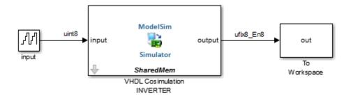
The model contains an HDL Cosimulation block (labeled "VHDL Cosimulation INVERTER") simulating an 8-bit inverter that is enabled by an explicit clock. The inverter has a single input and a single output. The following sample shows VHDL code for the inverter:
