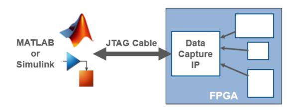
You can choose between two workflows to capture data from your FPGA board and return it to MATLAB or Simulink.
