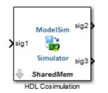
You configure an HDL Cosimulation block by specifying values for parameters in a block parameters dialog box. The HDL Cosimulation block parameters dialog box consists of tabbed panes that specify the following information:
