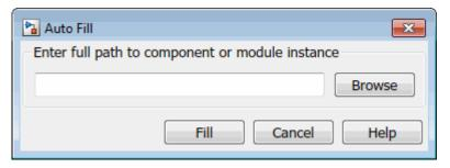
This modal dialog box requests an instance path to a component or module in your HDL model; here you enter an explicit HDL path into the edit field. The path you enter is not a file path and has nothing to do with the source files.
