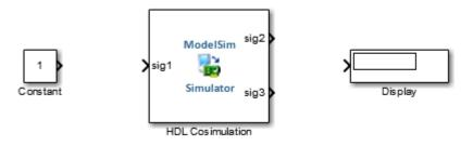
Next, configure the Constant block, which is the model's input source, by performing the following actions:
