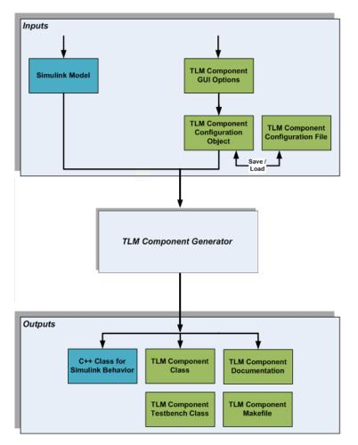
After code generation is complete, you can then use these generated files (outputs) to create the standalone TLM executable. See "Export TLM Component" on page 25-2.
