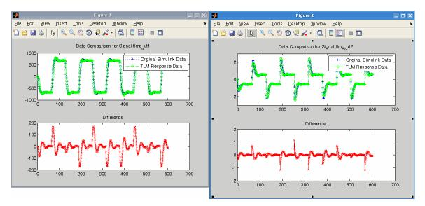
This difference occurs because the Simulink signal capture necessarily makes the signals discrete and thus the same exact data is not used in both the Simulink and stand-alone SystemC simulations. You can improve the fidelity of the discrete signal simulation in SystemC by choosing a smaller fundamental step size in Simulink before clicking **Verify TLM Component**.
