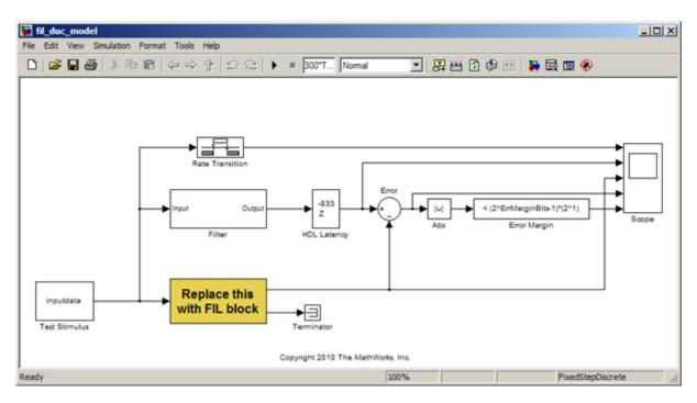
2. Double-click the FIL block to open the block mask. Click **Load** to program the FPGA with the generated programming file.
