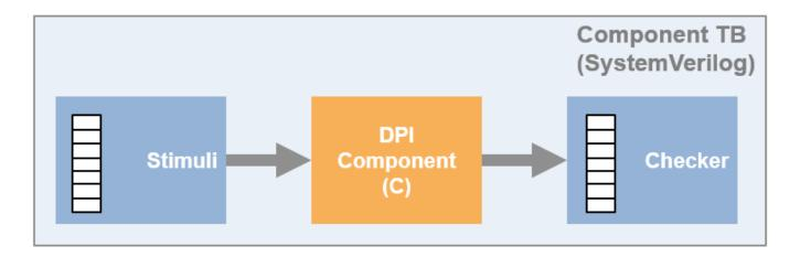
If you enable logging on test points in your model, the generated test bench also compares their signal values in the SystemVerilog component with logged values from Simulink.
