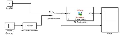
The model contains an HDL Cosimulation block (labeled HDL\_Cosimulation1) simulating an 8-bit inverter that is enabled by an explicit clock. The inverter has a single input and a single output. The following code excerpt lists the Verilog code for the inverter:
