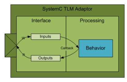
To control the architecture of the generated TLM component, you can choose among several options. Incorporating a memory map is one of the most effective options. The following figure demonstrates the behavior of a generated TLM component with a full complement of features enabled.
