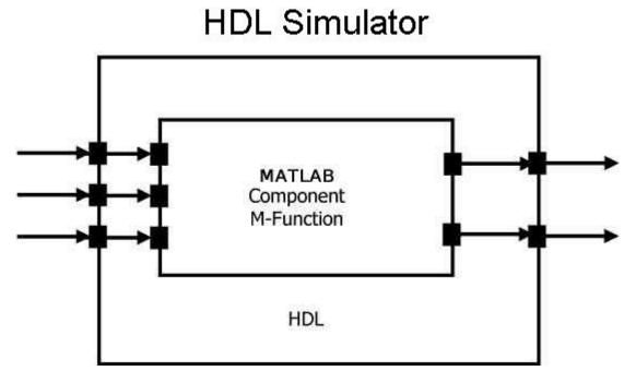
When linked with MATLAB, the HDL simulator functions as the client, with MATLAB as the server. The following figure shows a multiple-client scenario connecting to the server at TCP/IP socket port 4449.
