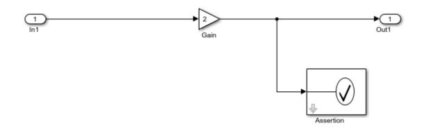
This example uses the Assertion block to monitor the Gain output and return a warning when the signal is zero. Double-click the Assertion block to configure its parameters. Set **Severity** to
